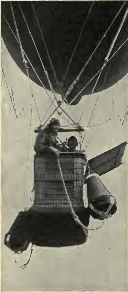
[Official photograph.] KITE BALLOON WITH PARACHUTES ATTACHED.
